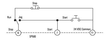
Selecting jog by an externally supplied switch will effectively turn the start pushbutton into a jog pushbutton. Jog speed will be the most recent set reference.
