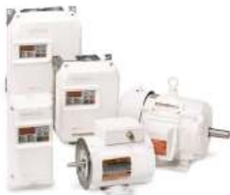
*Reliance® Electric's SP500 controller is a compact, low-cost AC PWM inverter that is designed and built in North America. Utilizing state-of-the-art digital microprocessing concepts and IGBT (insulated gate bi-polar) transistors, SP500 offers "trip-free" adjustable-speed performance for AC induction and synchronous motors.*
