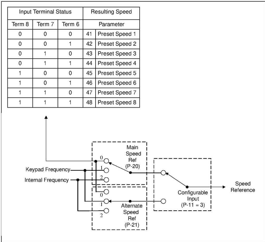
Figure 7.2 – Speed Reference Source for Model B Drives
