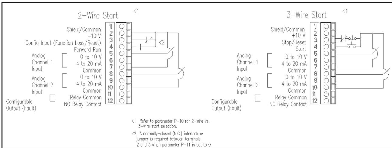
Figure 5.4 – Model C Control Signal Terminal Block Wiring
