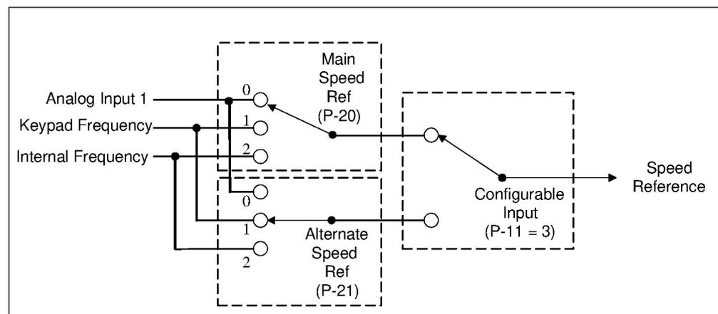
Figure 7.1 – Speed Reference Source for Model A Drives
