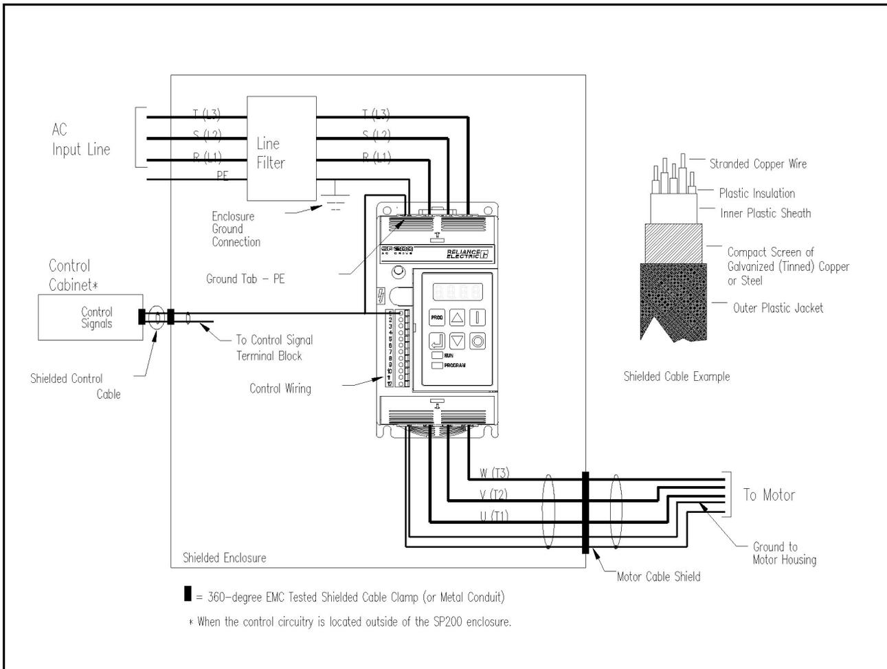
Figure C.1 – Grounding, Control, and Motor Connections
