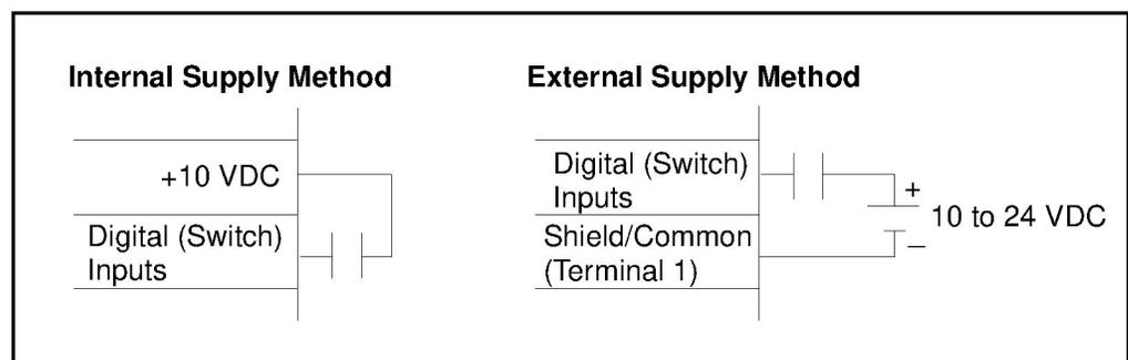
Figure 5.1 – Supply Methods for Digital (Switch) Input Connections
