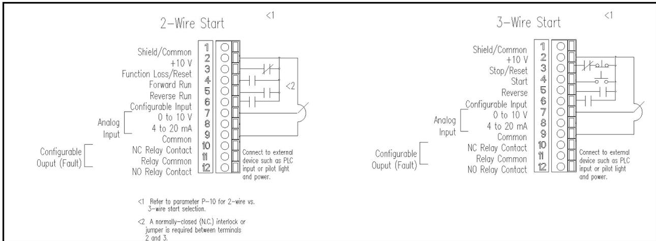
Figure 5.2 – Model A Control Signal Terminal Block Wiring
