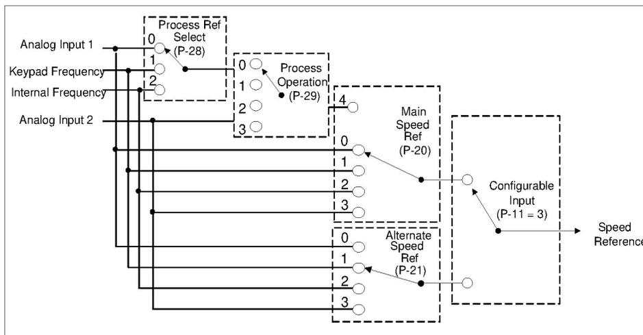
Figure 7.3 – Speed Reference Source for Model C Drives
