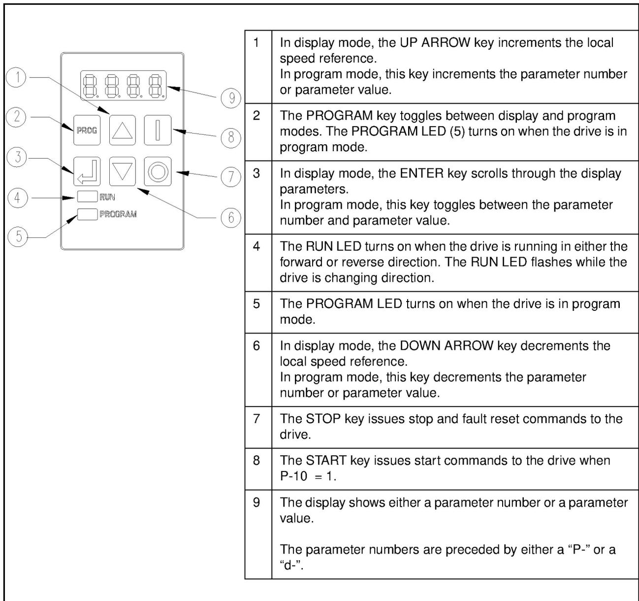
Figure 6.1 – Keypad Functions
