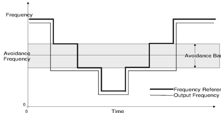
Note that the drive can accelerate and decelerate through the avoidance band. However, it cannot operate at a steady state within the avoidance band. Setting the value of this parameter to zero disables the avoidance frequency feature.
