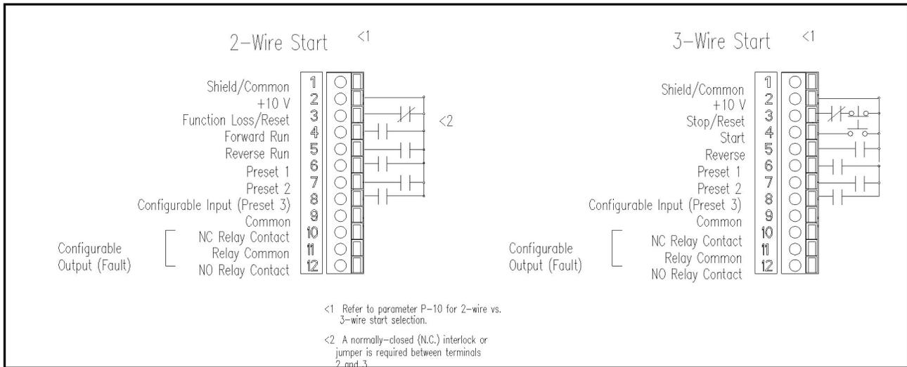
Figure 5.3 – Model B Control Signal Terminal Block Wiring
