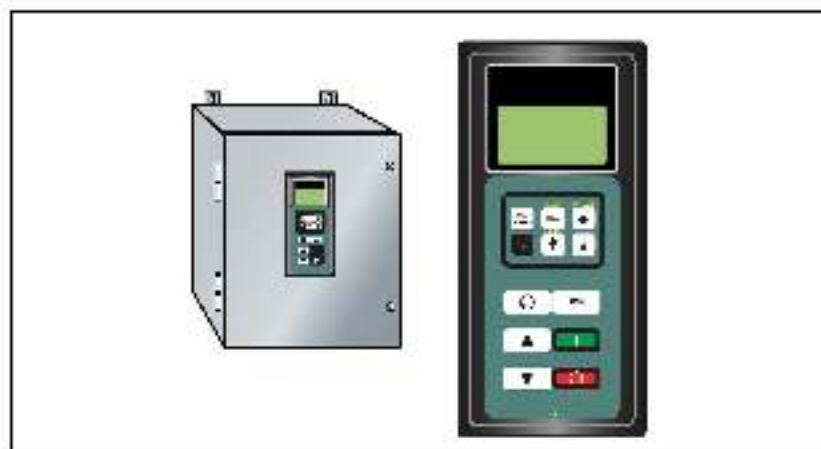
Figure 2 – MD4LCD-PNL or MD4ALCD OIM Mounted to Cabinet
