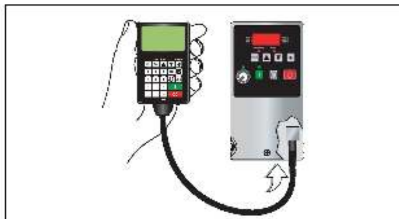
Figure 1 – MD1CC OIM Connected to an MD60 AC Drive
