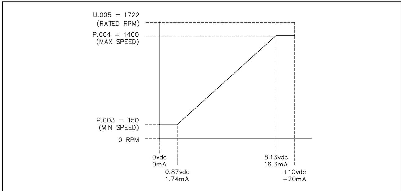
**Figure 6.2 - Relationship of Analog Input Speed Reference to Minimum and Maximum Speed**
