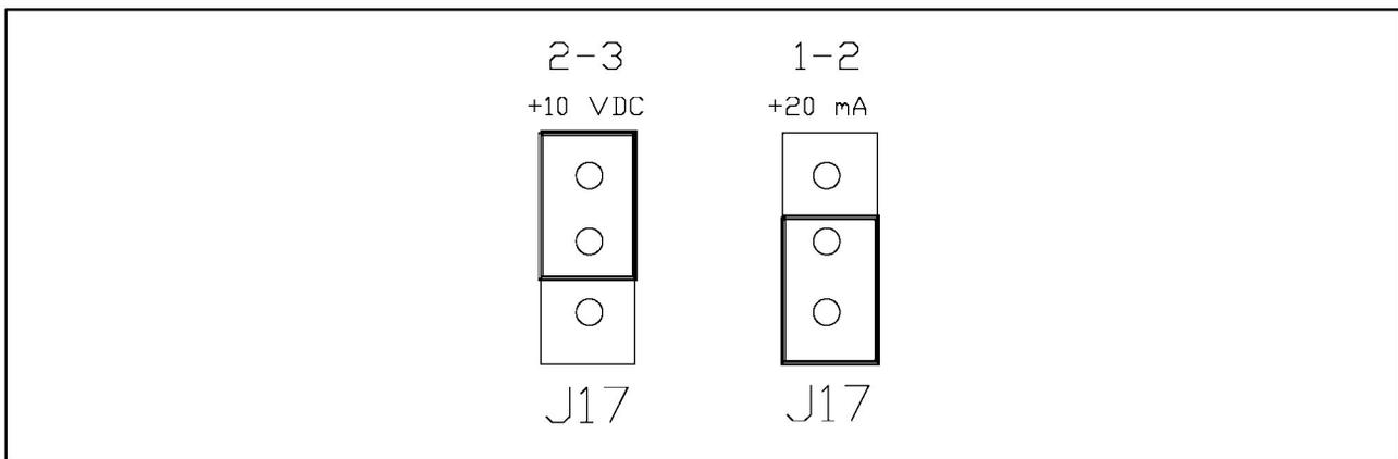
Figure 3.11 - Analog Output Jumper Setting (J17)
