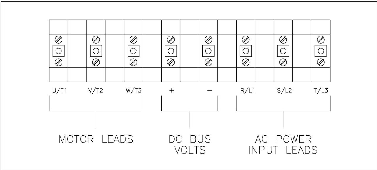
Figure 3.8 - Power Terminal Strip Wiring (460 VAC 15 and 20 HP)
