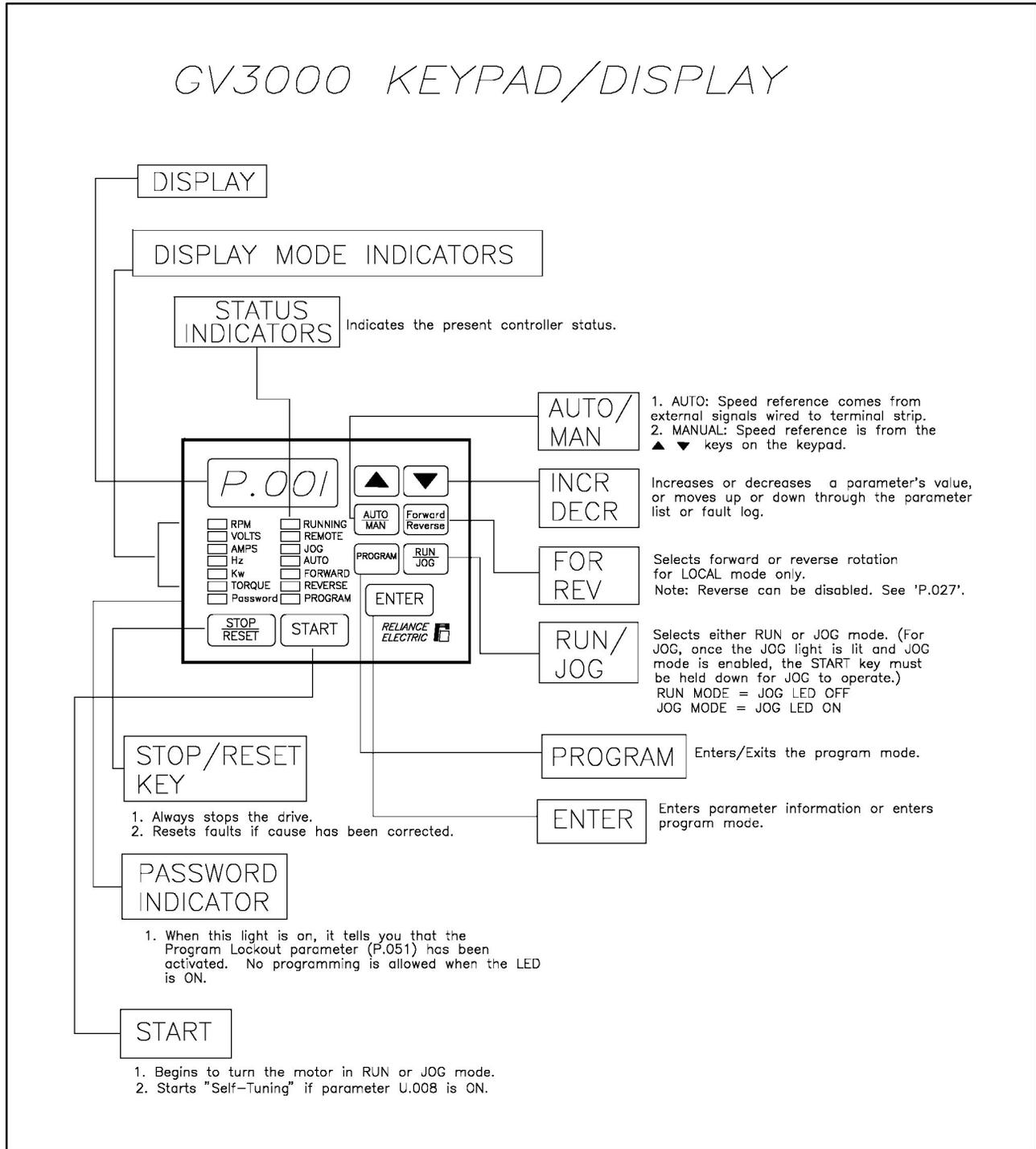
Figure 4.1 - GV3000 Front Panel Keypad/Display
