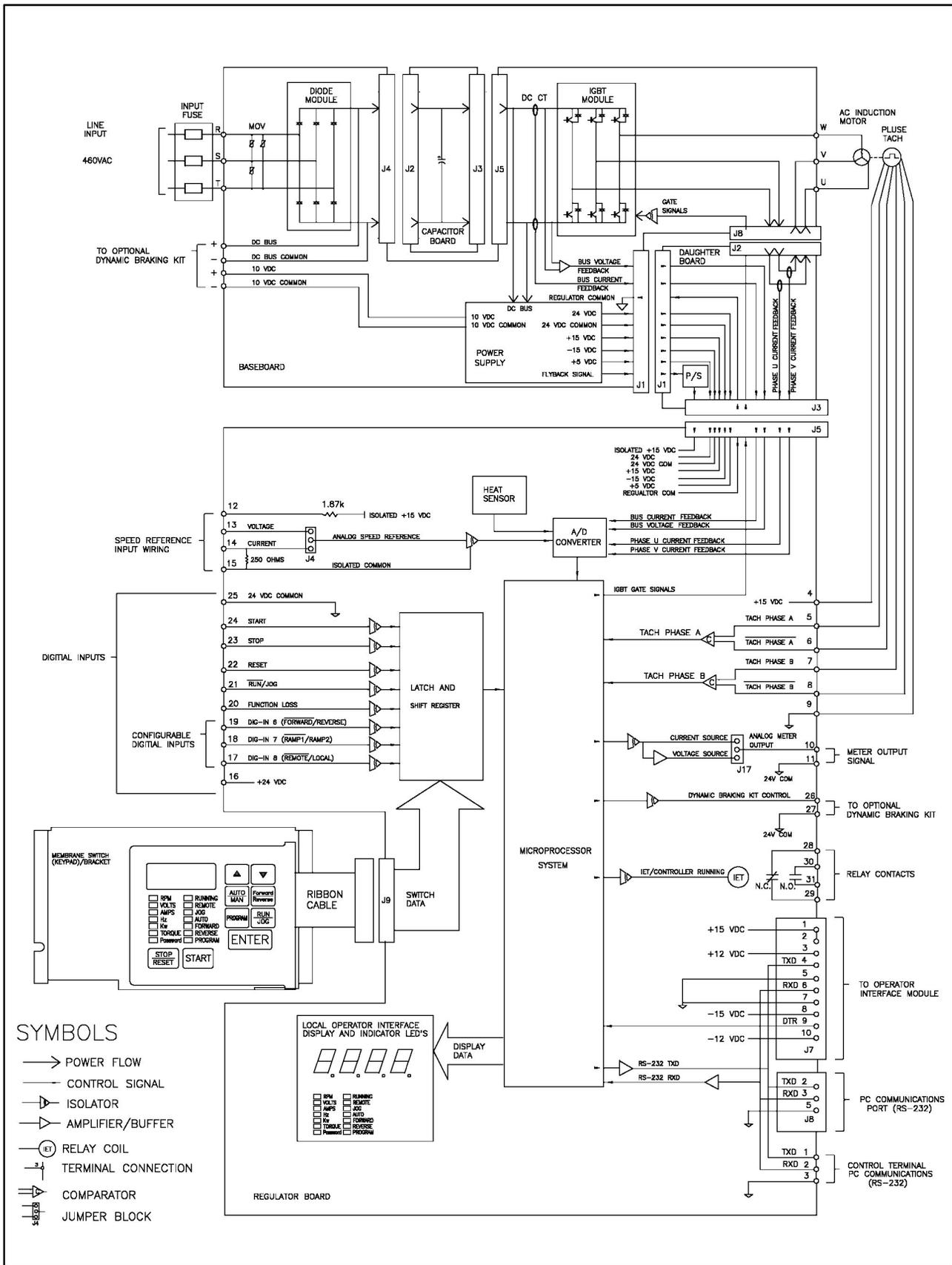
Figure 7.2 - Typical System Block Diagram
