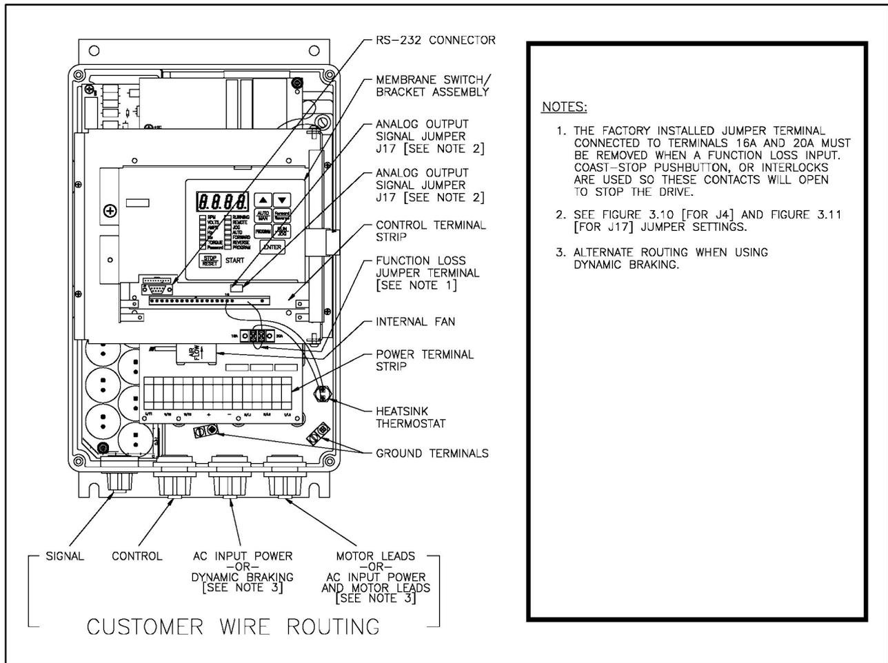
Figure 3.6 - GV3000 Wiring Locations (460 VAC 15 and 20 HP)
