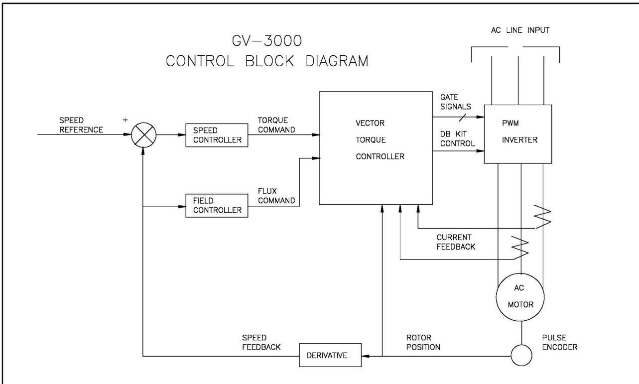
Figure 7.1 - Block Diagram of the GV3000 Vector Control
