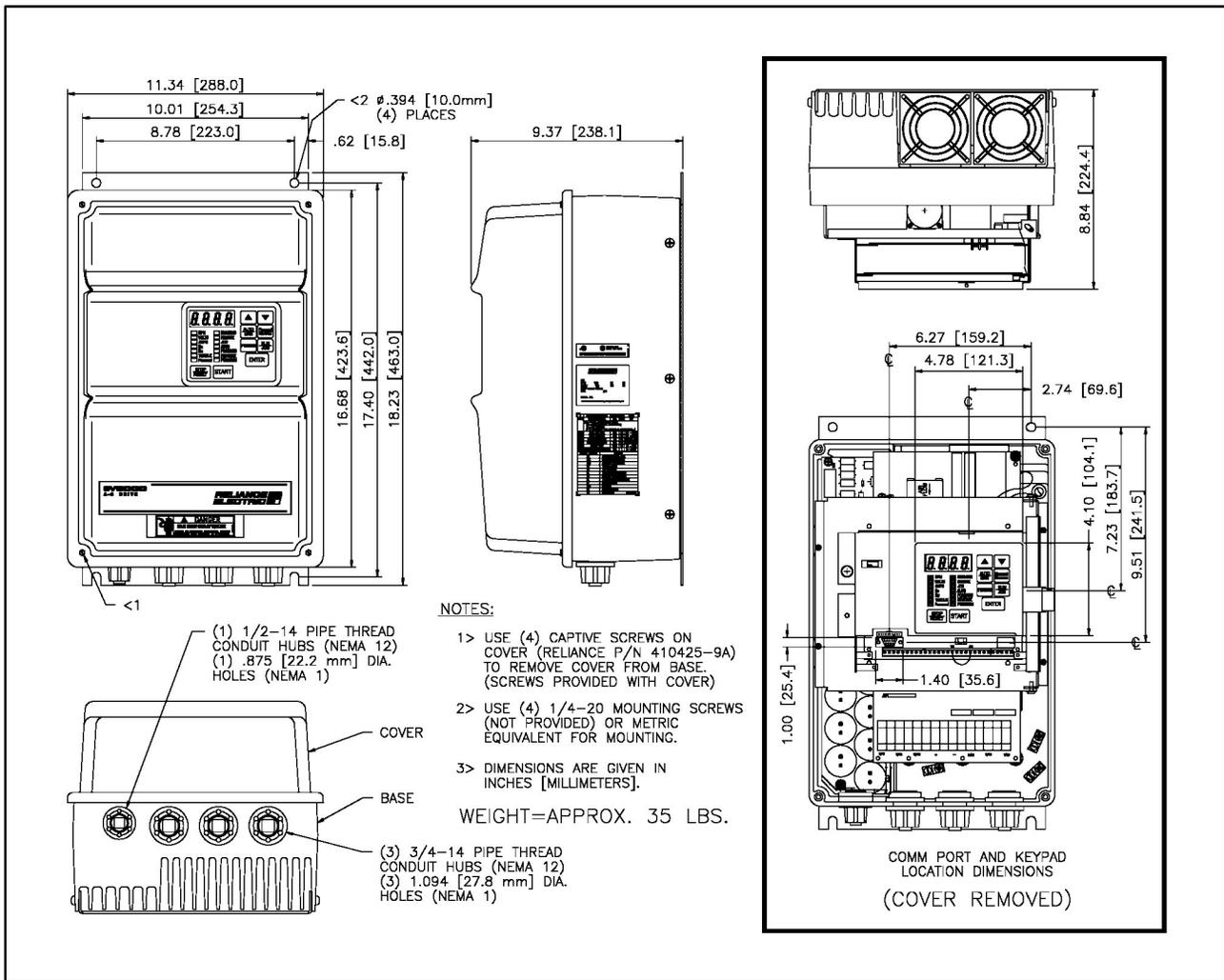
Figure 3.3 - GV3000 Drive Physical Dimensions (460 VAC 15 and 20 HP)
