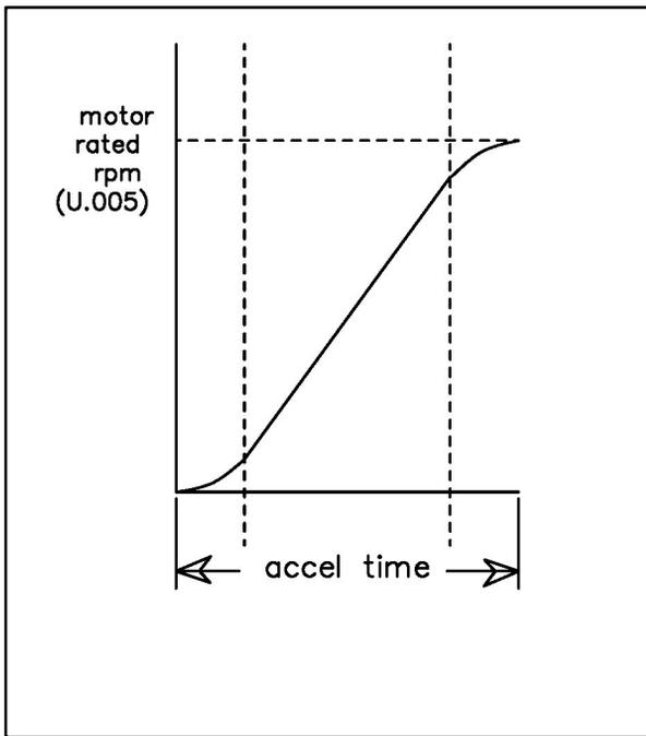
Figure 6.5 - S-Curve Acceleration
