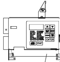
MEMBRANE SWITCH (KEYPAD)/BRACKET
