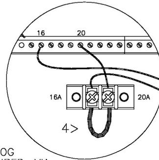
ALL CUSTOMER WIRING COMES IN AT THE BOTTOM OF THE CONTROL TERMINAL STRIP
