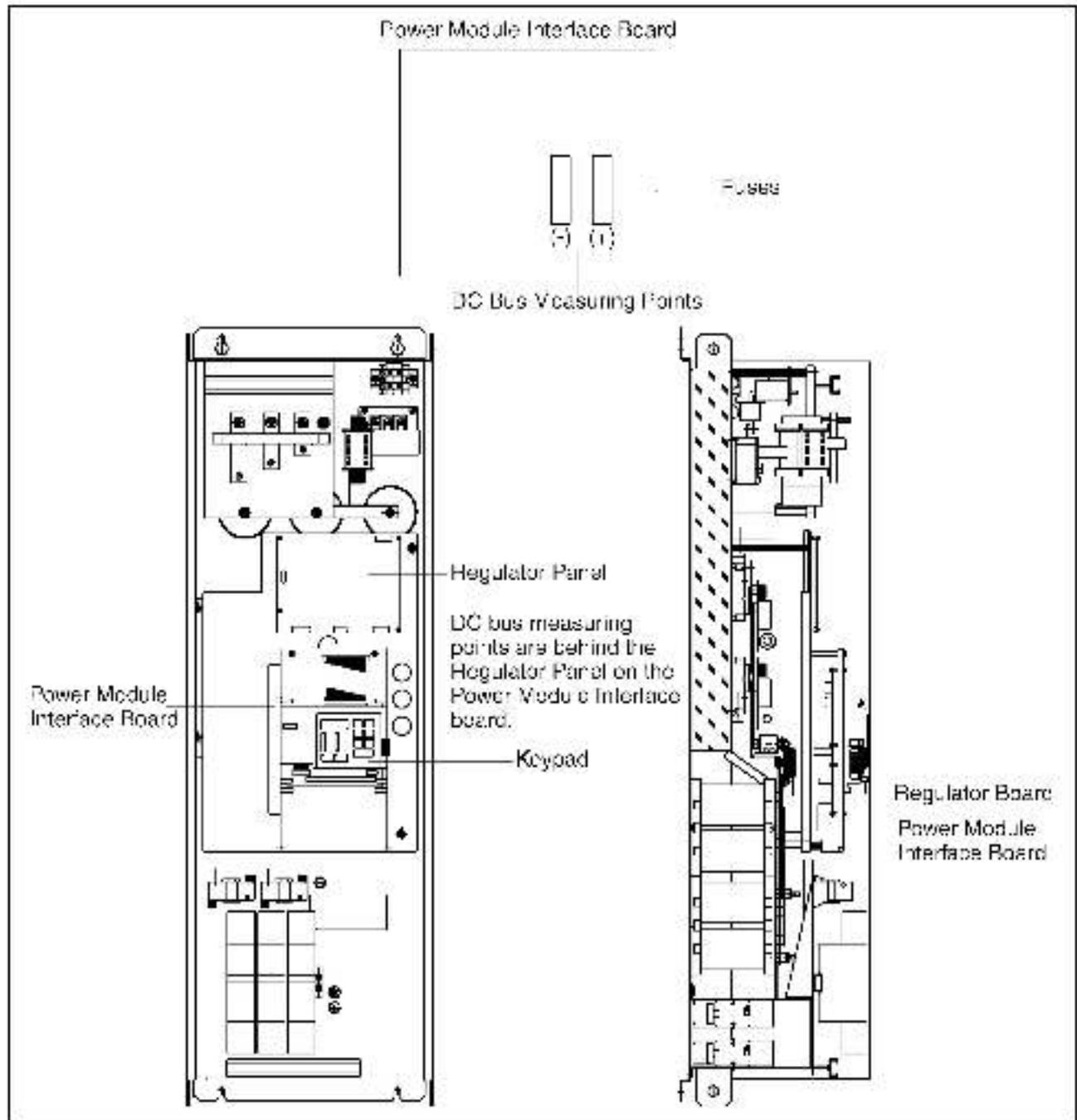
Figure 2.17 – 100 to 150 HP Drive Components and Locations
