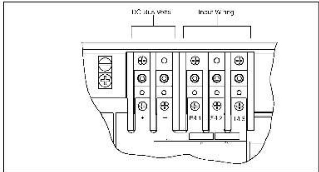
Figure 2-11 – DC Bus Voltage Terminals (25 to 60 HP & 480VAC)
