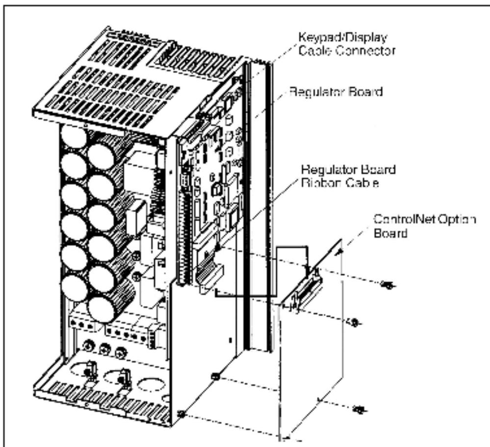
Figure 2-20 – Installing the ControlNet Option Board
