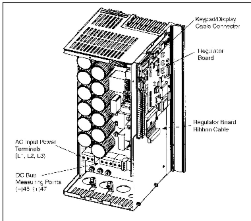
Figure 2-13 – 24 to 50 Amp GV3300/SH Rockshell Drive (Cover and Front Panel Removed)
