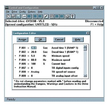
From the "File Menu", drive configurations can be created, opened, saved, and printed. Once a file has been opened it can be downloaded to the drive. Configurations can be saved as files for future use or as a permanent record. This makes it simple to duplicate configurations for drives on repeat applications.
