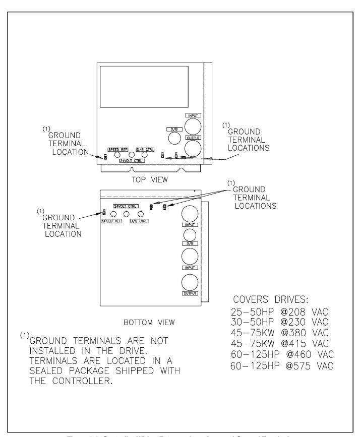
Figure 3-2. Controller Wiring Entrance Locations and Ground Terminals.
