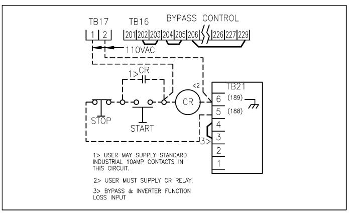
Figure 4-13. Three-Wire, 110VAC Internal Supply, Start/Stop Wiring.
