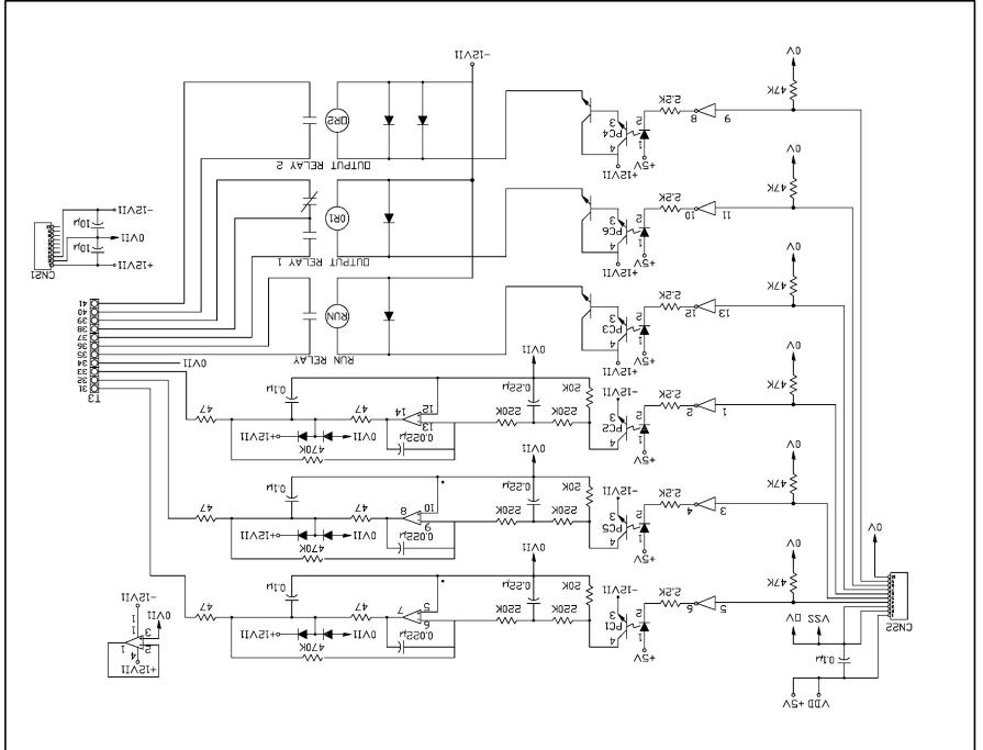
Figure 7-3. Remote Meter Interface Card Circuit Diagram.
