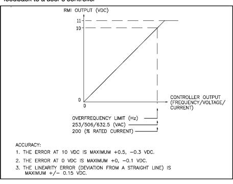
Figure 7-1. Optional Remote Meter Interface Card Output Characteristics.
