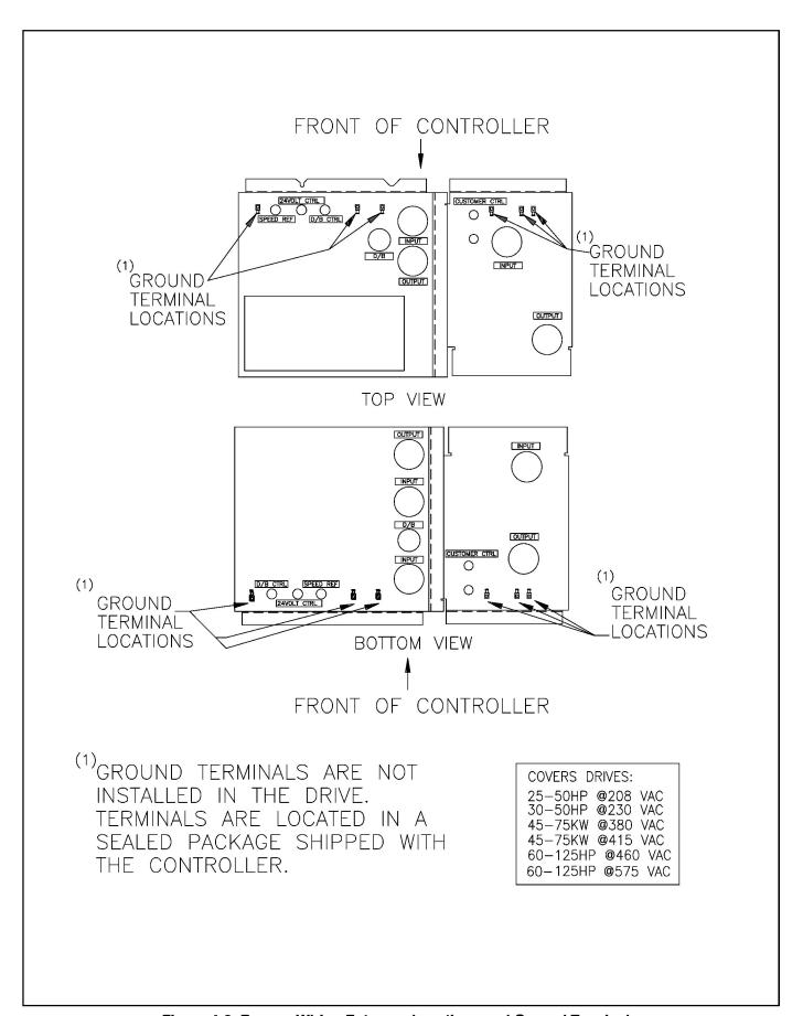
Figure 4-2. Bypass Wiring Entrance Locations and Ground Terminals.
