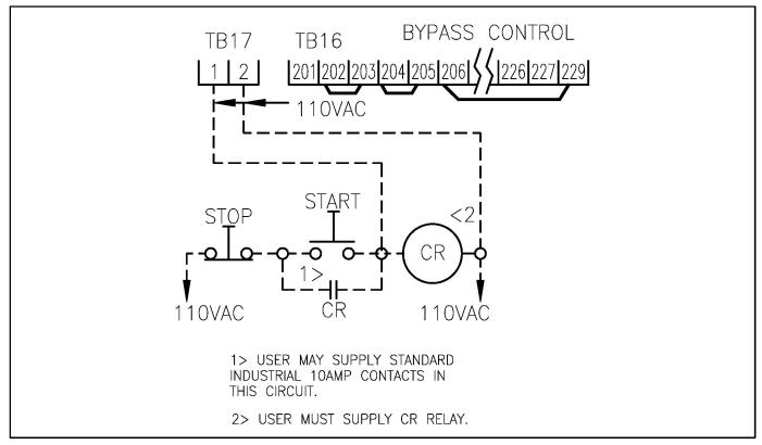
Figure 4-14. Three-Wire, 110VAC Customer-Supplied, Start/Stop Wiring.
