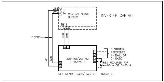
Figure 7-6. Gain/Bias Reference Adjustment Kit Wiring.
