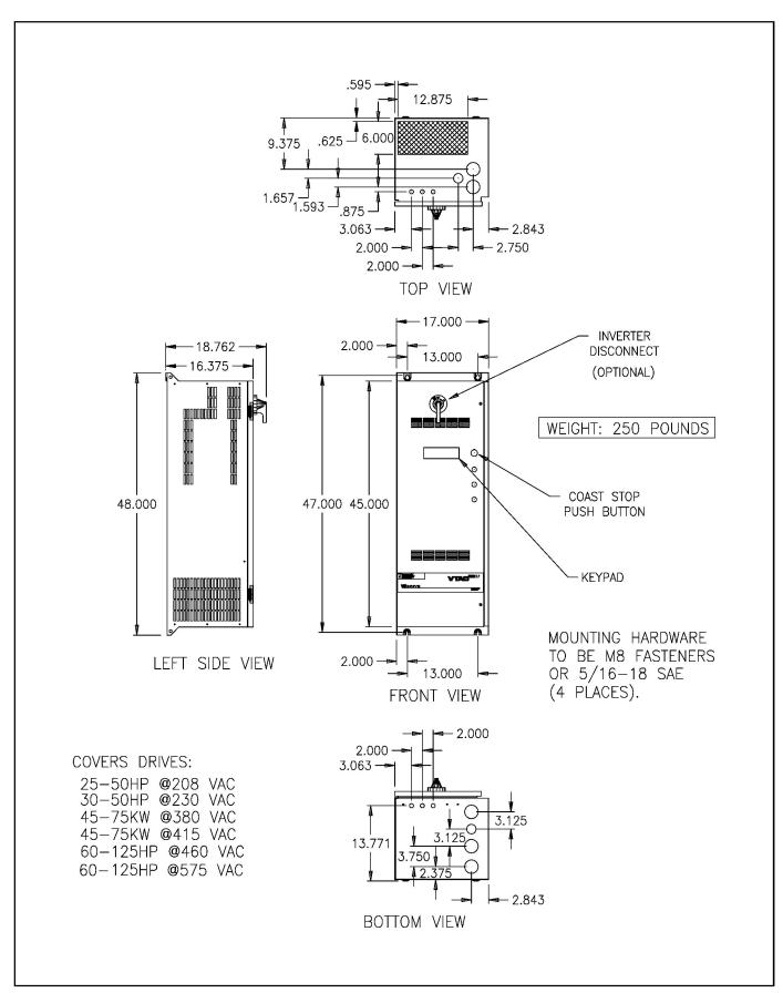
Figure 3-1. Physical Dimensions (Inverter Only).
