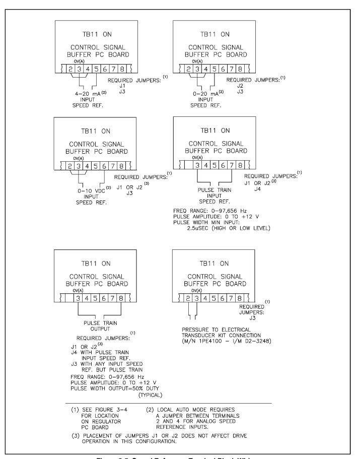
Figure 3-5. Speed Reference Terminal Block Wiring.
