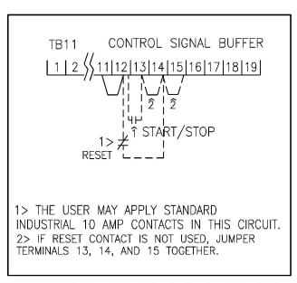
Figure 3-11. 24 VDC (Two-Wire, Single Contact) Start/Stop Wiring.
