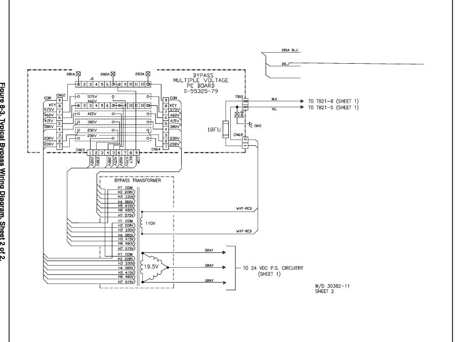
Figure 8-3. Typical Bypass Wiring Diagram, Sheet 2 of 2.
