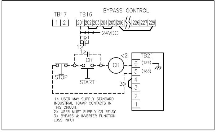
Figure 4-12. Three-Wire, 24VDC Start/Stop Wiring.
