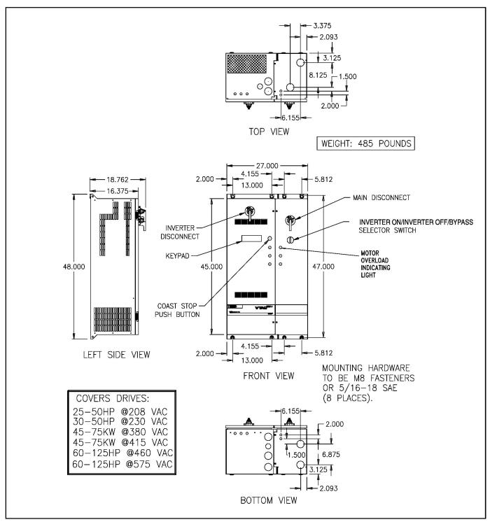
Figure 4-1. Bypass Physical Dimensions (with Inverter Section).
