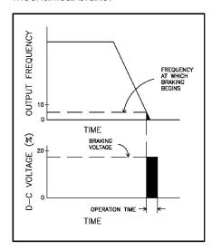
Figure 6-12. D-C Braking Operation.
