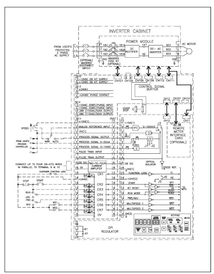
Figure 3-6. Control Signal Buffer Board Functional Block Diagram.
