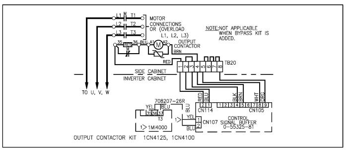
Figure 7-8. Output Contactor Kit 1CN4125, 1CN4100.
