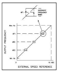
Figure 6-10. Avoidance Frequency Operation.
