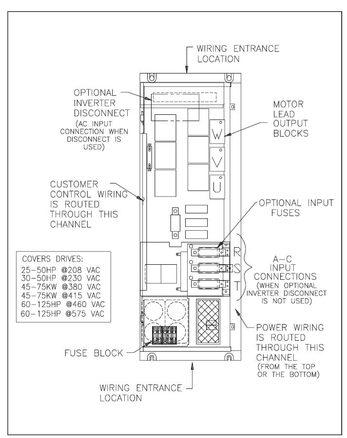
Figure 3-3. Typical Input/Output Power Wiring Locations (Inverter Only).
