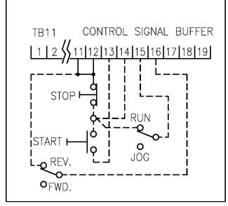
Figure 3-12. 24 VDC (Three-Wire) Start/Stop Wiring.
