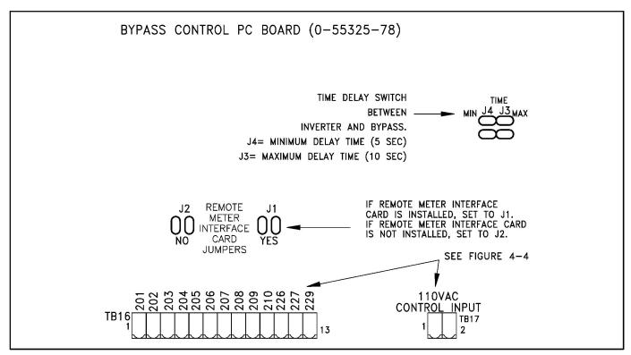
Figure 4-5. Bypass Control Board.
