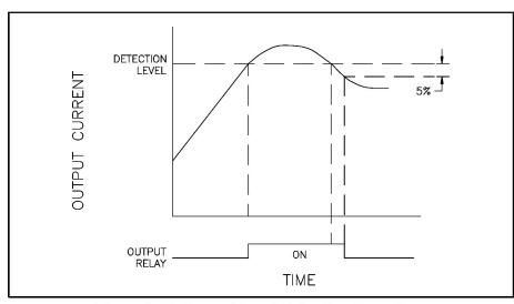
Figure 6-15. Current Level Detection Operation.
