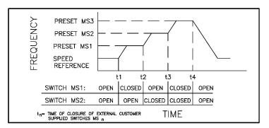
Figure 6-9. Typical Multi-Speed Preset Application.
