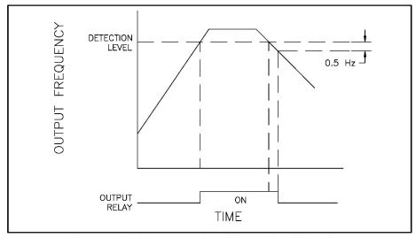
Figure 6-14. Frequency Level Detection Operation.
