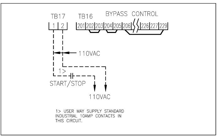
Figure 4-11. Two-Wire, Single-Contact, 110VAC Customer-Supplied, Start/Stop Wiring.
