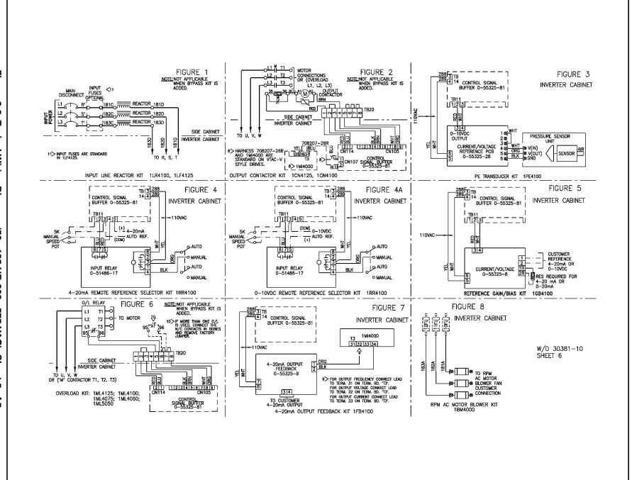
Figure 8-2. Typical Wiring Diagram (50-125 HP, 208-575 VAC). Sheet 5 으 Ģ
