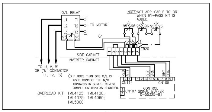
Figure 7-4. Motor Overload Kit Wiring.
