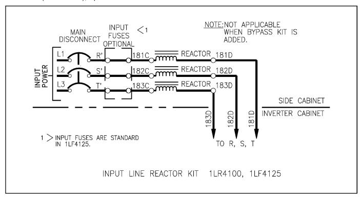
Figure 7-7. Input Line Reactor Kit 1LR4100, 1LF4125.
