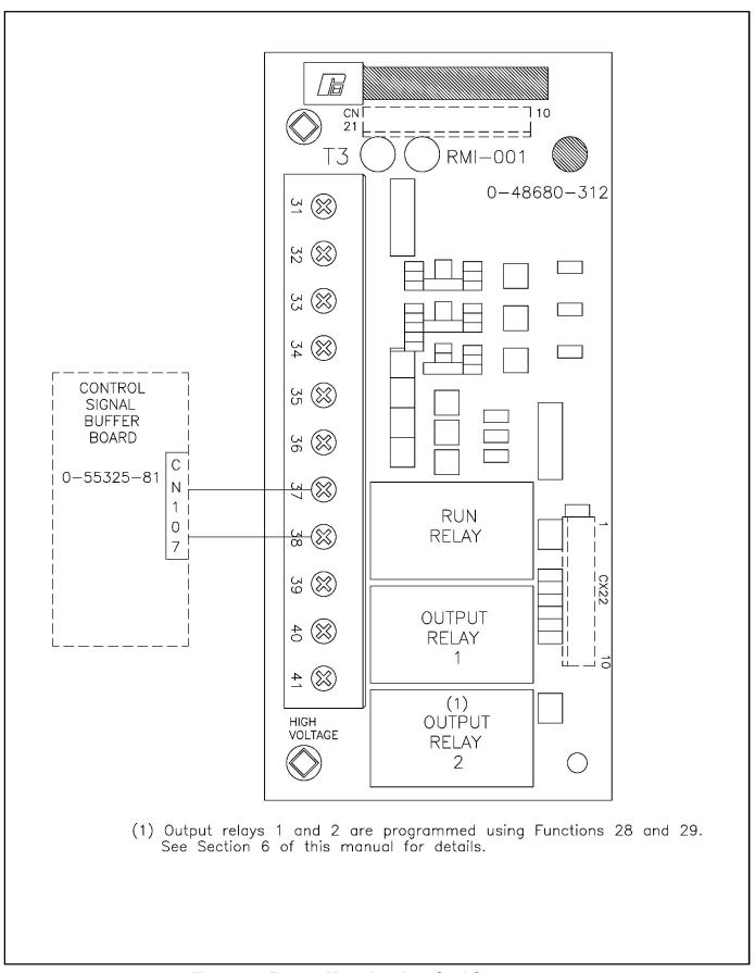
Figure 7-2. Remote Meter Interface Card Components.
