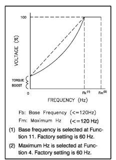
Figure 6-11. Variable Torque Curve
