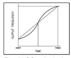
Figure 6-7. S-Curve Acceleration.
