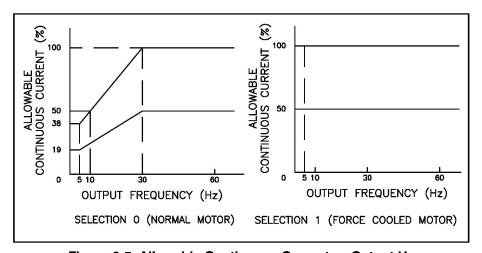
Figure 6-5. Allowable Continuous Current vs Output Hz (with Function 13 at 50% and 100% Settings).
