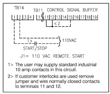
Figure 3-9. Customer-Supplied 110 VAC (Two-Wire, Single Contact) Start/Stop Wiring.
