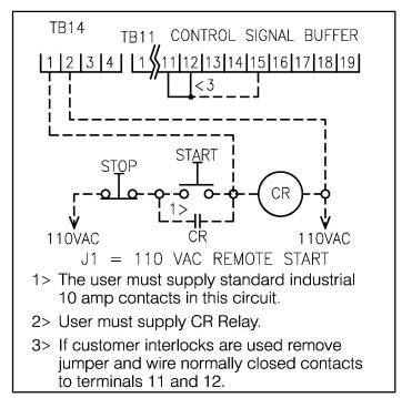
Figure 3-10. Customer-Supplied 110 VAC (Three-Wire) Start/Stop Wiring.
