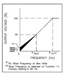
Figure 6-2. Manual Torque Boost Adjustable Range (Constant Torque shown).
