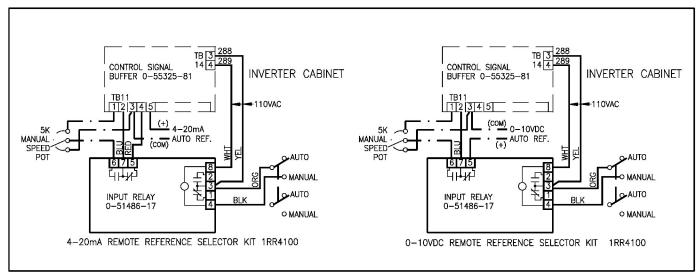
Figure 7-5. Remote Reference Selector Kit Wiring.
