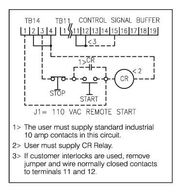
Figure 3-8. 110 VAC (Three-Wire) Start/Stop Wiring Using Internal Supply.
