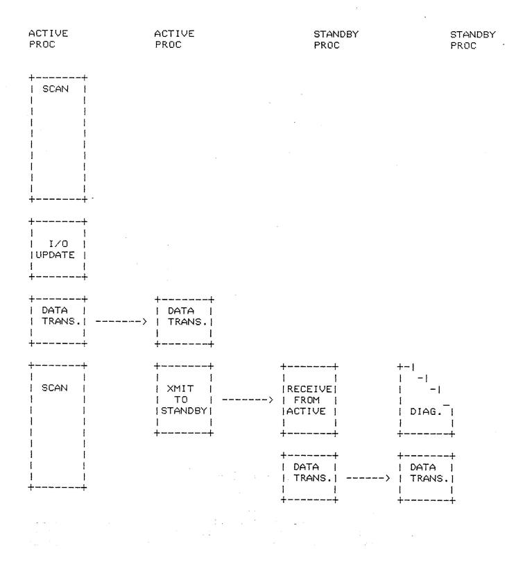
Figure 2 Example Timing Diagram of Data Transfer
