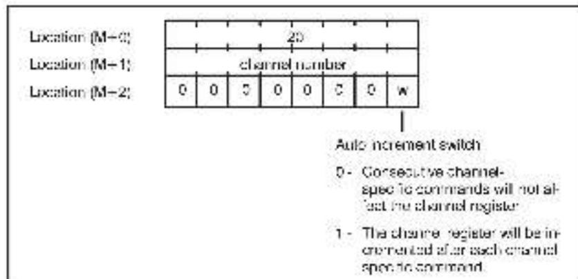
Valid channel numbers range from 0 to 15, corresponding to channels 0-15.
