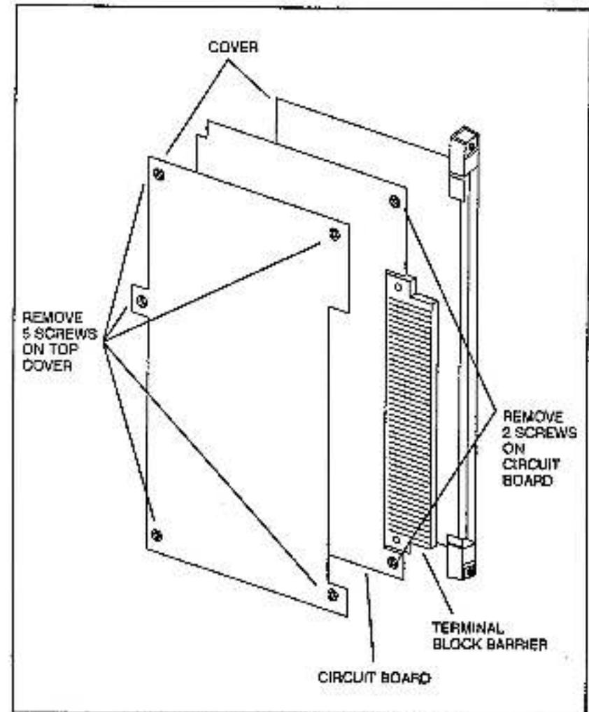
Figure 5.0 - Disassembling the Module for Calibration
