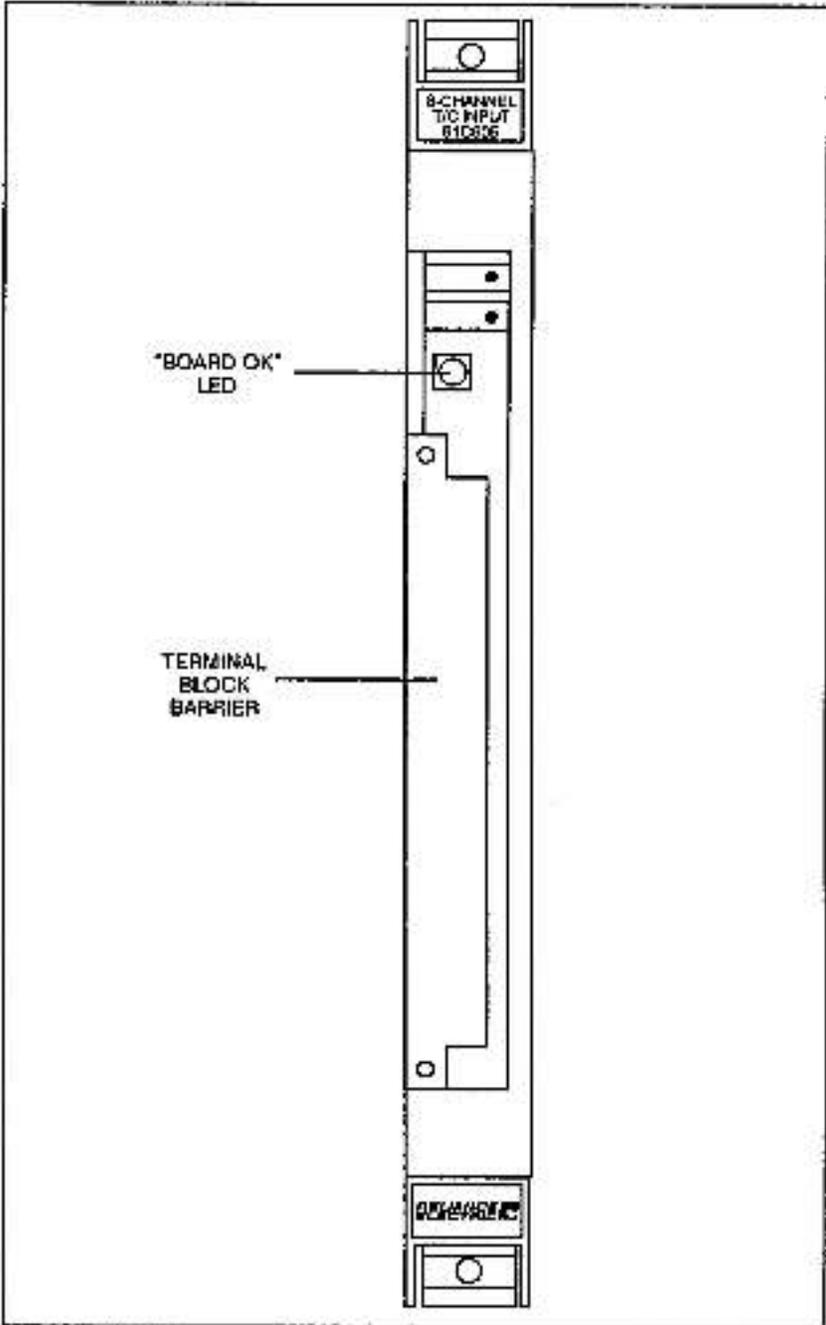
Figure 2.0 - Eight-Channel Isolated Thermocouple Input Module Faceplate
