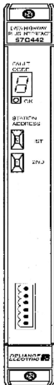
Figure 2.2 Data Highway Plus Interface Module Front Panel
