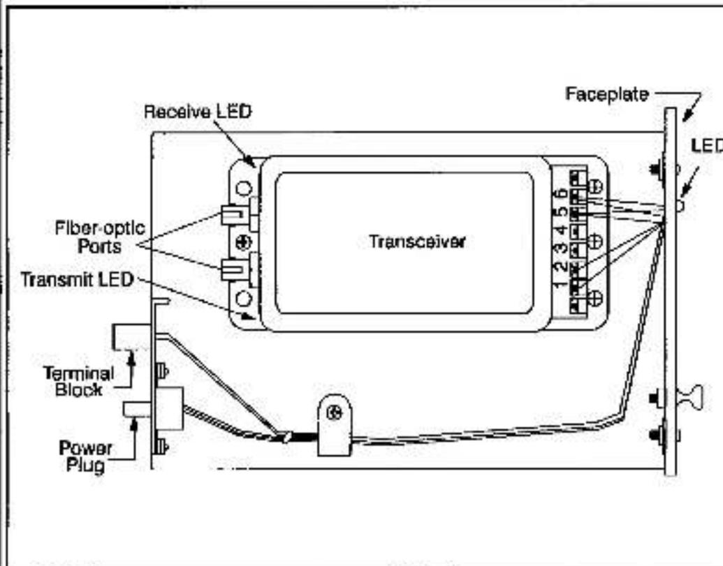
Figure L1.6 - Rack-Mounted Transceiver
