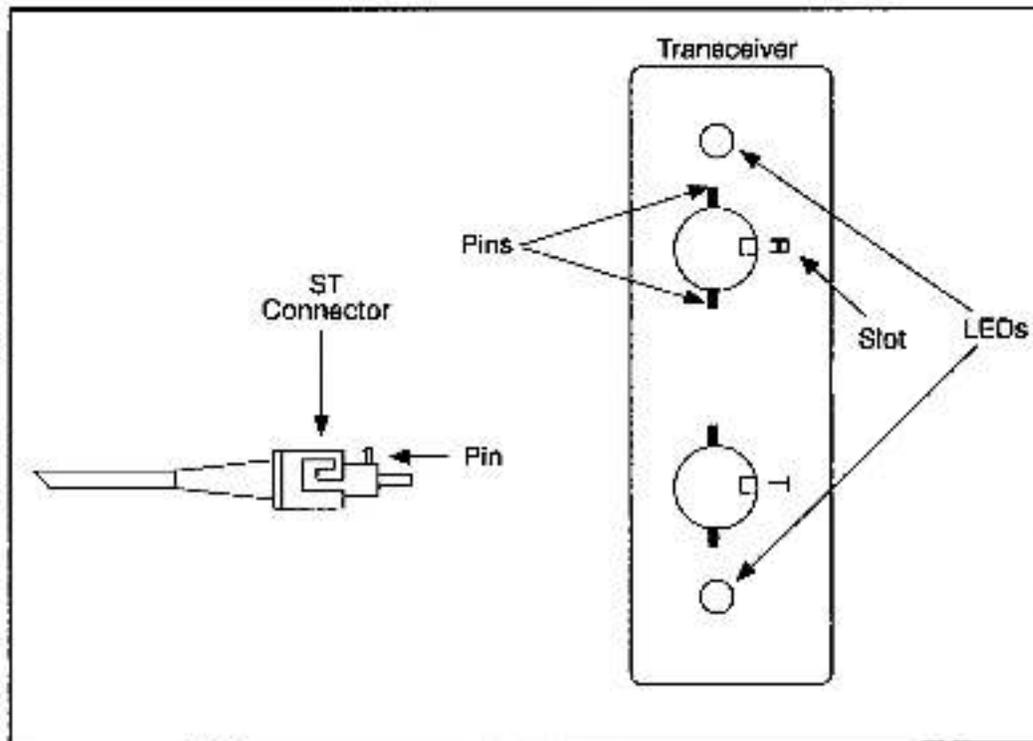
Figure L2.8 - Fiber-Optic Ports and Connectors
