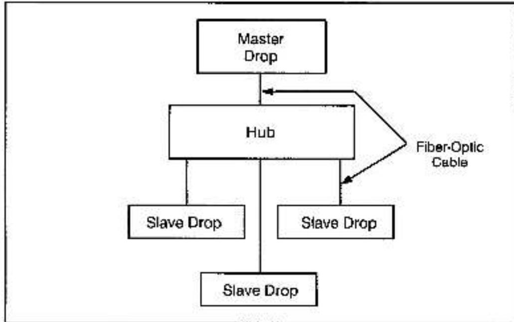
Figure 1.2 - A Typical DCS-NET Fiber-Optic Cable Network Layout
