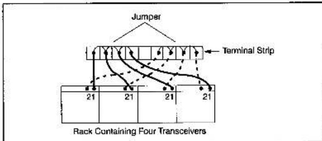
Figure L2.5 - Connecting Rack-Mounted Transceivers to a Terminal Strip
