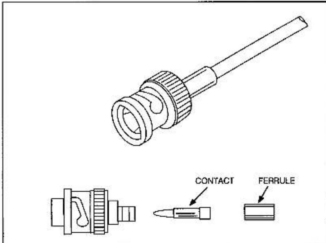
Figure 3.4 - Dual Crimp BNC Plug Connector
