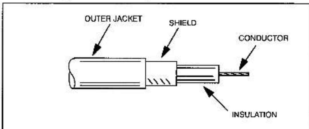
Figure 3.3 - Coaxial Cable
