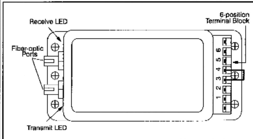
Figure L1.4 - Stand-Alone Transceiver
