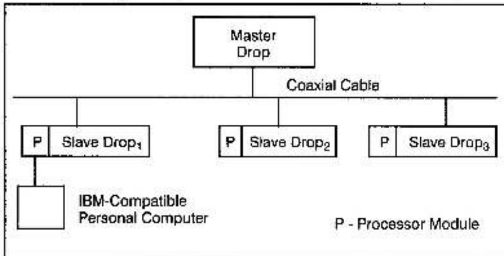
Figure 1.4 - Programming Terminal Communication Example (Coax)
