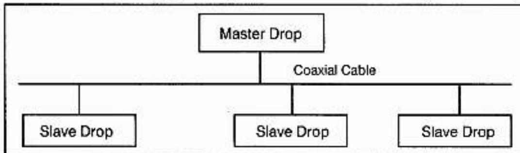
Figure 1.1 - A Typical DCS-NET Coaxial Cable Network Layout
