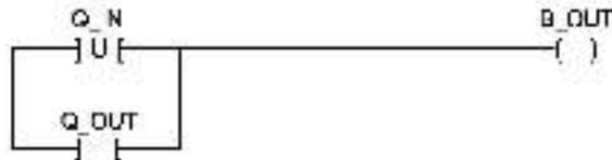
If Q\_IN is on when the sequence is inserted, B\_OUT will turn on. If a different bit in the word where Q\_IN is defined was already used by the task, then B\_OUT will not turn on until Q\_IN turns off and then on again.
